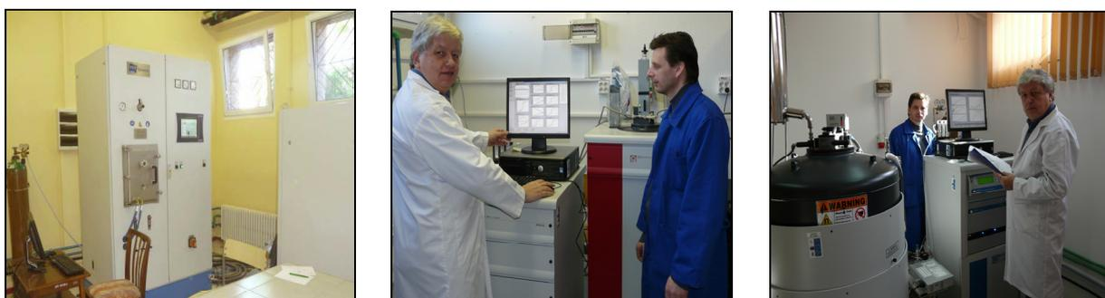
*Spark Plasma Sintering (left), MPMS (middle) and PPMS (right) systems*
