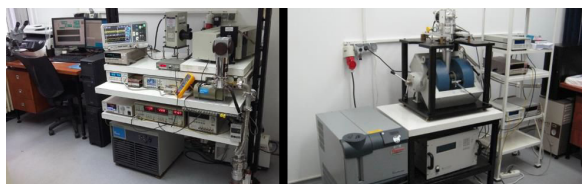
Set-ups for electrical (including ferroelectric & charge storage) and photoelectrical measurements (left); Hall effect and magnetoresistance measurements (right).
