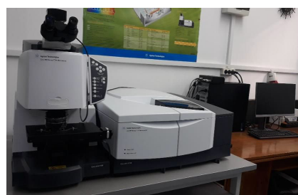
Infrared spectro-microscope, Cary 600 from Agilent Technologies
