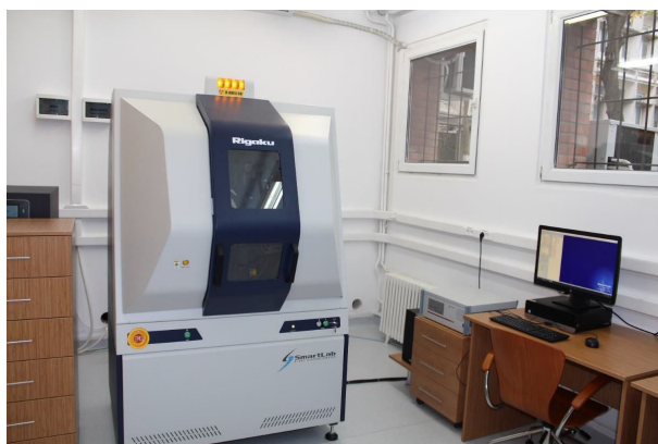
Fig. 3. XRD equipment for thin film characterization, produced by Rigaku.
