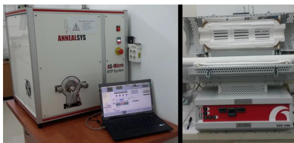
Rapid thermal processing - RTP system (left); Three independent temperature zone horizontal split tube furnace (right).
