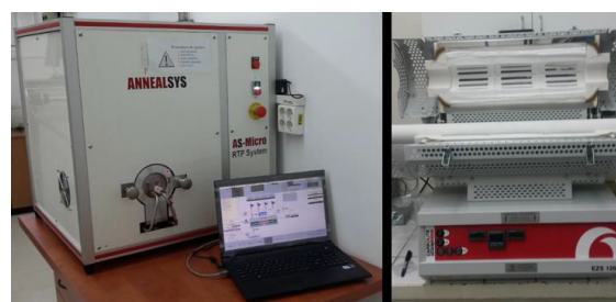
Rapid thermal processor (left); horizontal split tube furnace with 3 independent temperature zones (right)
