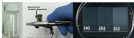
Fig. 1. Three different g\text{-C}_3\text{N}_4 films prepared by spray deposition on FTO substrates. The codes of the prepared and characterized samples are listed in Table 1.
