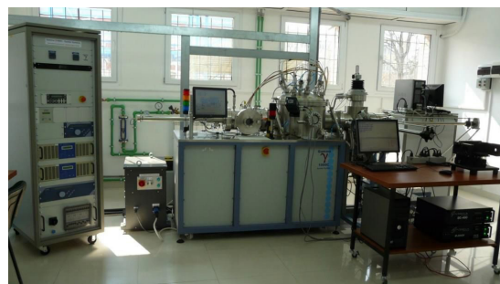
Magnetron sputtering equipment equipped with in situ AES and LEED techniques, allowing also real time in situ ellipsometric monitoring.
