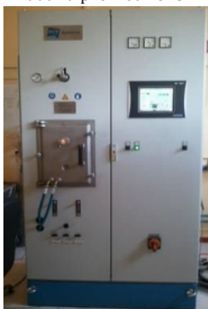
Spark PLASMA sintering plant used to obtain high density bulk materials.
