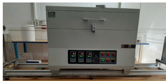
Physical Vapor Transport equipment for transition metal dichalcogenides
