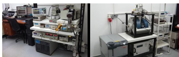
Set-ups for electrical and photoelectrical measurements (left); Hall effect and magnetoresistance measurements (right).
