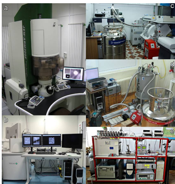
a. High resolution analytical transmission electron microscope (0.08 nm in mode STEM HAADF);
