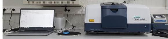
**Fig. 3b** FTIR spectroscopic platform with extended NIR – MID – farIR spectral range, 12000 – 50  $\text{cm}^{-1}$ .
