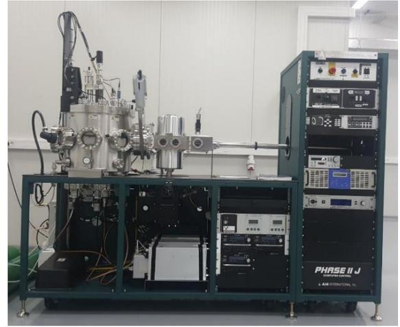
**Fig. 1b** RF, DC and p-DC magnetron sputtering system, AJA PHASE II, for the deposition of semiconductor thin films.
