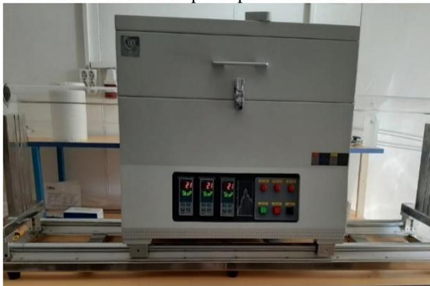
Physical Vapor Transport equipment for transition metal dichalcogenides
