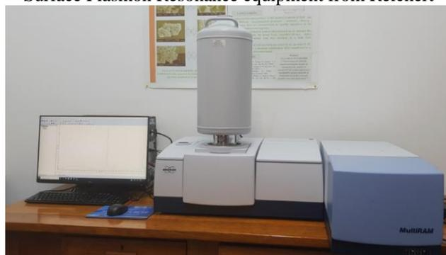
MultiRam FTIR Raman spectrophotometer from Bruker
