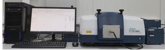
Spectrometru FTIR, model JASCO (NEAR & MID IR)
