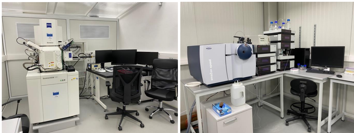
Left – high resolution SEM Gemini 500; right - liquid chromatograph with mass spectrometer.
