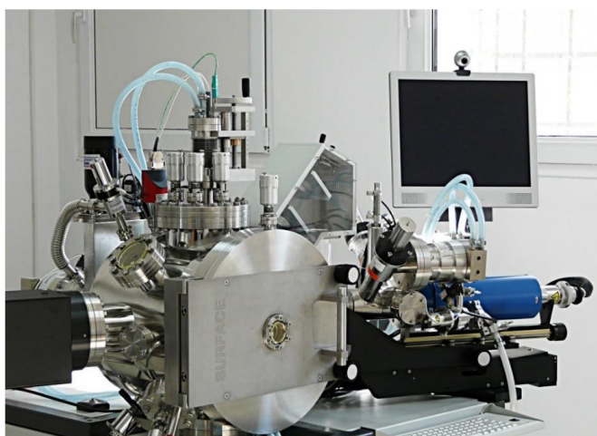
Fig. 1a PLD workstation assembly, SURFACE & SCIENCE systems+technology GmbH, for the deposition of ferroelectric thin films.
