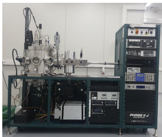
Fig. 1b RF, DC and p-DC magnetron sputtering system, AJA PHASE II J, for the deposition of semiconductor thin films.
