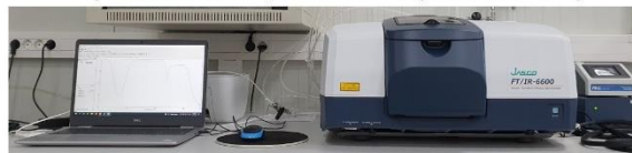
Fig. 3b FTIR spectroscopic platform with extended NIR – MID – farIR spectral range, 12000 – 50 cm -1 .
