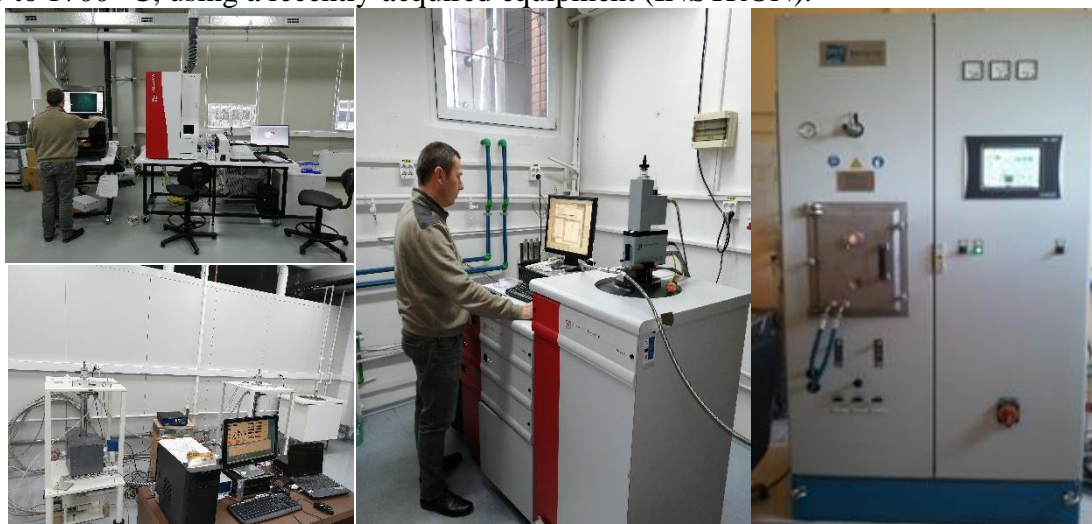
ICP-MS with LA for thin films (upper left), Mossbauer spectrometers with closed circuit He cryostats (lower left) and SQUID device – Quantum Design, of high sensitivity (middle). Spark plasma sintering plant (FCT Systeme GmbH) used to obtain high density bulk materials (right).
