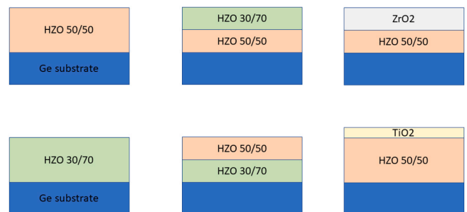
Fig. 1. Schematic representation of the configuration of the simple layers and of the multilayers used.
