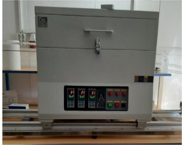
**Fig. 60–4** Physical Vapor Transport equipment for transition metal dichalcogenides.
