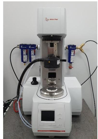
**Fig. 20–2b** ANTON PARR MCR302e modular rheometer.
