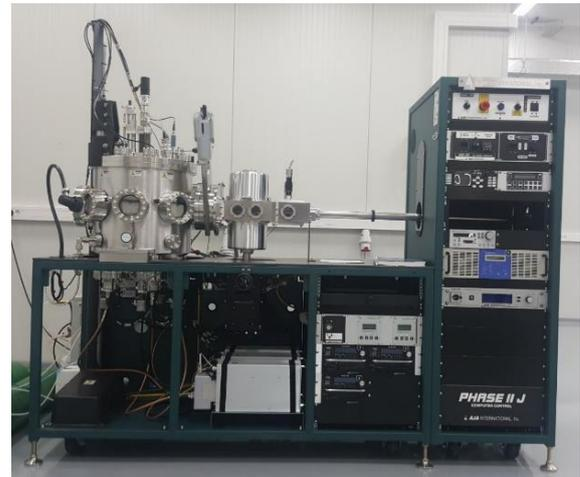
**Fig. 20–1b** RF, DC and p-DC magnetron sputtering system, AJA PHASE II, for the deposition of semiconductor thin-films.
