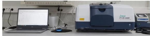
**Fig. 20–3b** FTIR spectroscopic platform with extended NIR – MID – farIR spectral range, 12000 – 50 cm<sup>-1</sup>.
