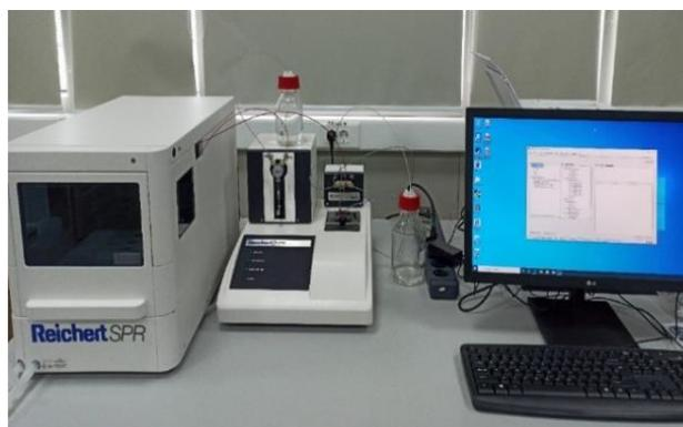
**Fig. 60–2** Surface Plasmon Resonance equipment from Reichert.
