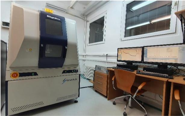
**Fig. 20–3a** RIGAKU SmartLab 3 kW high-resolution XRD system for thin-films analysis.
