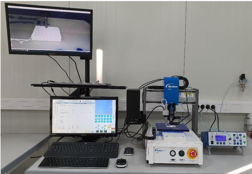
**Fig. 20–2a** 3D printing system by robocasting (direct ink writing) technology, NORDSON EFD, EV series, with Ultimius V dispenser.
