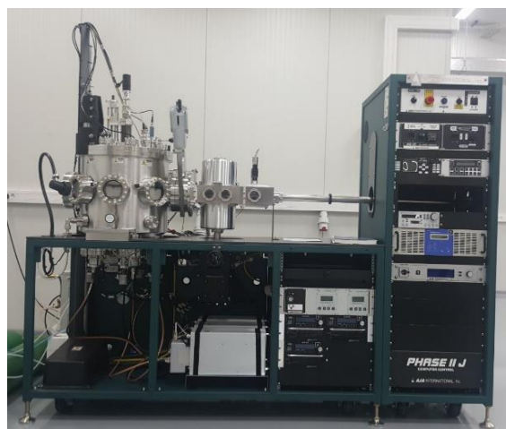
Fig. 20-1b RF, DC and p-DC magnetron sputtering system, AJA PHASE II, for the deposition of semiconductor thin-films.
