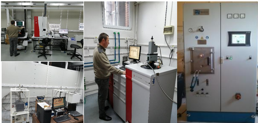
Fig. 30-1 ICP-MS with LA for thin-films (upper left), Mossbauer spectrometers with closed circuit He cryostats (lower left) and SQUID device – Quantum Design, of high sensitivity (middle). Spark plasma sintering plant (FCT Systeme GmbH) used to obtain high density bulk materials (right).
