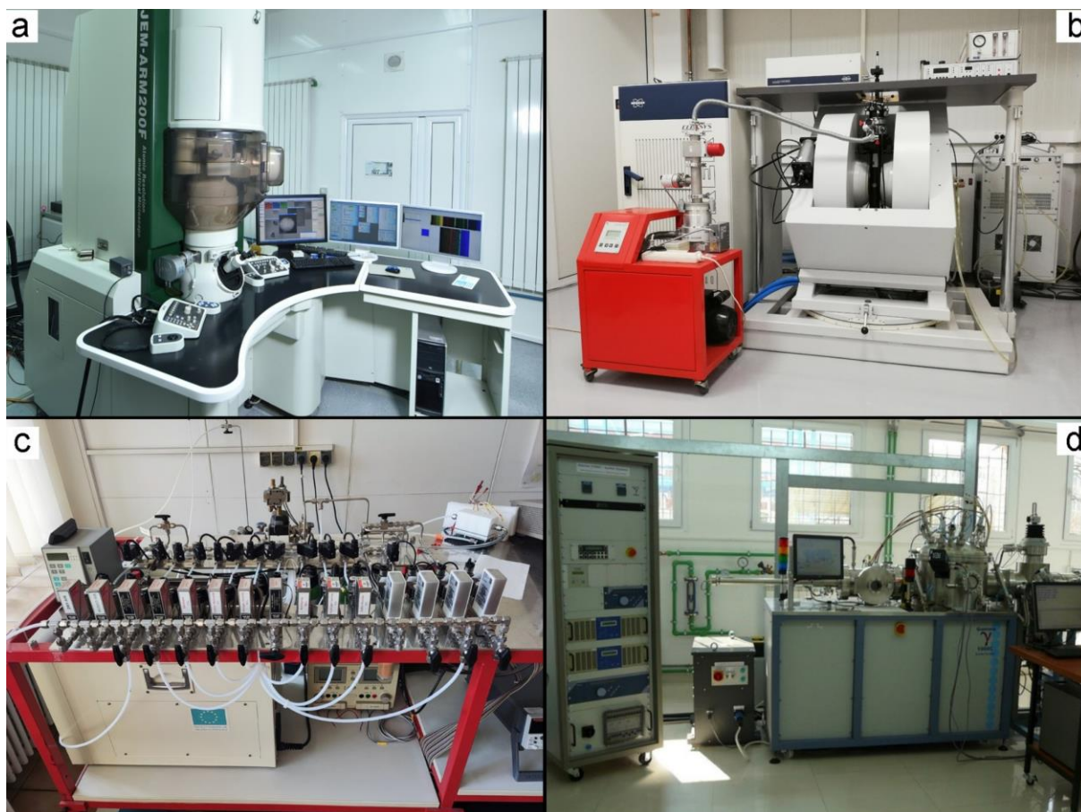
Fig. 70-1 (a) JEM ARM200F aberration-corrected analytical transmission electron microscope; (b) Bruker EPR spectrometer in CW Q-band with ENDOR accessory; (c) Setup for electrical measurements under controlled atmosphere gas mixing station; (d) Magnetron sputtering installation for thin-films deposition, equipped with in situ AES, LEED, and ellipsometry.
