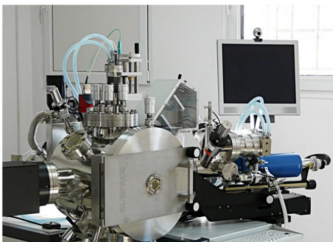
Fig. 20-1a PLD workstation assembly, SURFACE SCIENCE, for the deposition of ferroelectric thin-films.
