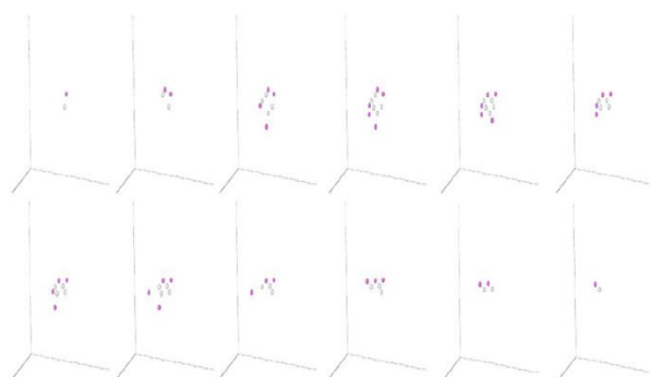
Figure 4. MD simulations of vacancy-interstitial pair production and recombination. V (grey) / I (magenta)
